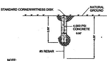
1. THE STANDARD CORNER/WITNESS DISK IS TO BE DRIVEN ON A 4.0' #5 REINFORCEMENT STEEL BAR (REBAR). THE BAR ASSEMBLY IS TO BE DRIVEN INTO THE CENTER OF A 6" DIA. x 2'-6" DEEP HOLE. THE HOLE IS TO BE FILLED WITH 4,000 PSI CONCRETE
